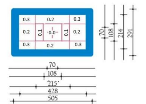
The two new lines are drawn across the trampoline bed from the current side tramlines using measurements as per the diagram.
